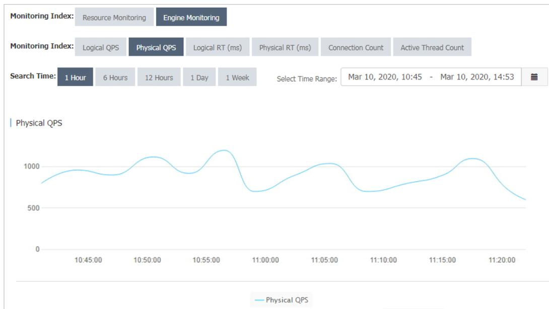
As shown in the preceding figures, logical QPS fluctuates between 80 and 150, and physical QPS fluctuates between 700 and 1,200.
