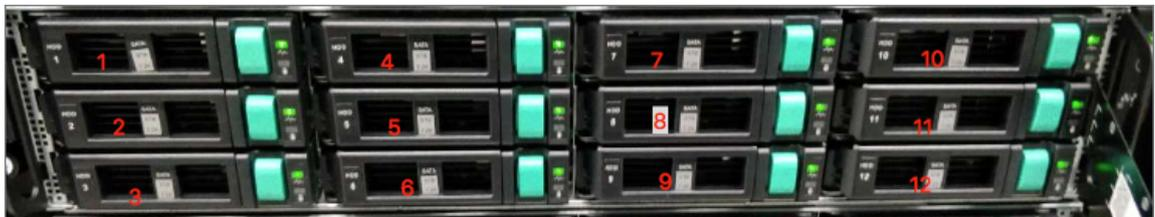
You should remove /dev/sdb1, that is, the hard disk in slot 1. Check that the SN of the hard disk is consistent with the SN found earlier.
